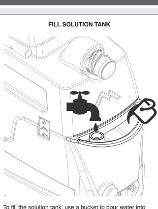
To fill the solution tank, use a bucket to pour water into the tank's opening located at the front of the unit. You can also use the easy faucet fill also located at the front of the unit. For best results, fill with warm water ( $140^{\circ}$  F).
