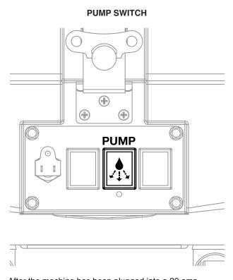
After the machine has been plugged into a 20 amp grounded outlet, turn on pump. Pull trigger on cleaning tool until tool releases a steady flow.
