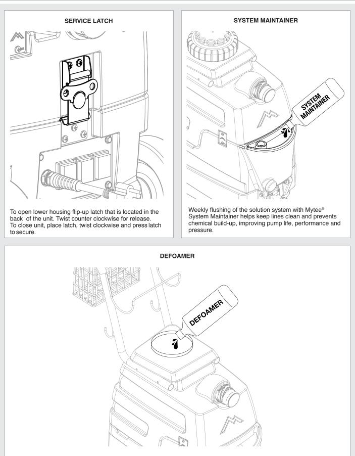
Add defoamer in the recovery tank to reduce foam, prolonging the life of the Mytee Lite™ vacuum motor.
