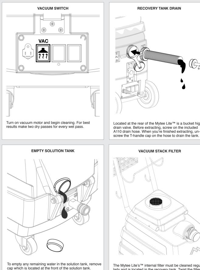
Located at the rear of the Mytee Lite™ is a bucket high drain valve. Before extracting, screw on the included A110 drain hose. When you're finished extracting, un-
