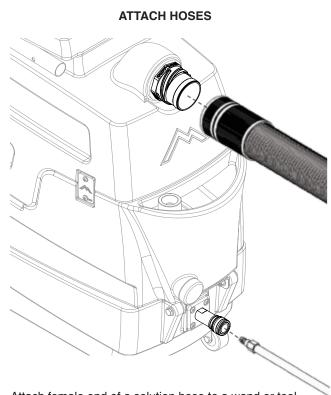
Attach female end of a solution hose to a wand or tool and the male end to the Mytee Lite's<sup>™</sup> QD. Then connect a vacuum hose to a wand and the male Cuff-Lynx<sup>™</sup> hose port.
