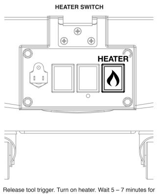
unit to pre-heat. Once heated, pull trigger on tool until hot water begins flowing.
